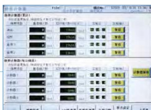
**冲头, 熔杯和维护计数器 Tip, sleeve, maintenance counter**
